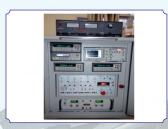
Function-This Test Rig has been designed and manufactured to meet the PIC requirements of Antiskid Controller Pt. No. 228700000 of HJT-36 aircraft.
