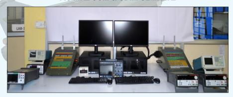
Servo Control Module (SCM) Test Jig is used for testing the Servo Control Module at SRU level with the help of PCB Interface Module which contains 196 Pin Airborne Connector for interacting between SCM Module and Test Jig. Test Jig Consist of test fixture test and monitoring point at the front panel and interface connector, for interface UUT (servo control module) with it. It also consists of workstation with DIO module and Respective driver software, used for simulation Digital module of AC Mk2
