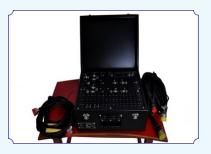
Function-The Centralised Warning System (CWS) test set is used on the aircraft to test the aircraft CWS. The test set can be used to test the CWS with or without the CWS related circuits (attention getters and lightening circuits).
