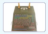
ASA test jig ASA sensor test jig. Acceleration sensor assembly (ASA) 3-Axis Test Jig (STTE) for measuring longitudinal, normal axis acceleration using ASA unit.
