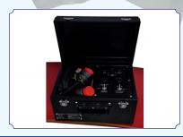
Function-The fuel dip system test box consists of test panel and cable stowage panel assembly, contained in a case. The fuel dip test box is used in conjunction with a digital timer to perform a series of static checks on the electrical circuits to the fuel dip systems.
