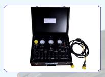
Function-The electrical power generation test set is designed for checking out the "dormant" circuits of the aircraft electrical power generation system and for checking voltage and frequency values at various points within the electrical generation system.
