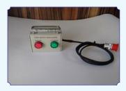
Function-During integration / testing the tow body commands bulbs are connected across the designed pin number to check the availability of particular signal as and when that particular command is initiated
