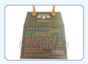
Function-AC Auxiliary Card Test Jig test Jig has provision to set certain signals in the UUT and to monitor all pins on the AC Auxiliary Card Test edge connector. The Fixture interfaces the cards to the appropriate power supplies, signal sources and monitoring devices like CRO, DMM and logic analyzer. Further provision is available to monitor activities on the various important pins. The power supplies are interfaced to UUT via
