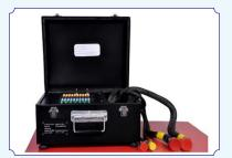
Function-The scope of the Break-in-Box is to monitor the voltage and current level at all the pins of ADR (Accident Data Recorder) and DAU (Data Acquisition Unit).
